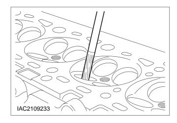
CAUTION: After reaming the valve guide, re-cut the valve seat as in Operation Number 21 231 9 and renew the valve.
