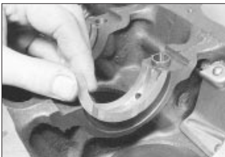
34.8 Removing a thrustwasher from the centre main bearing
