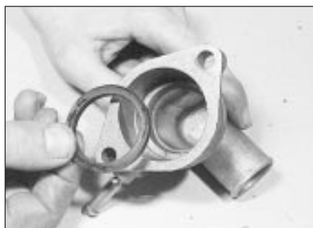
7.6c . . . and sealing ring
