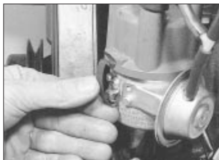
13.7 Securing distributor cap with spring clip - Bosch distributor
