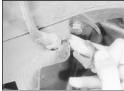
5.37 Removing a brake line securing clip from the suspension crossmember
