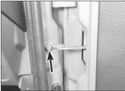
16.2 Remove the door check arm-to-body pillar bolt (arrowed)
