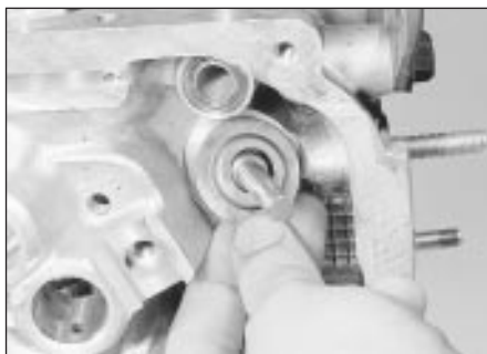
21.3a Remove the spring seat . . .
