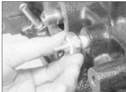
17.10 Removing the oil pressure warning lamp switch - 1.8 litre (R2A)
