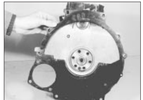
26.5 Withdrawing the engine adaptor plate
