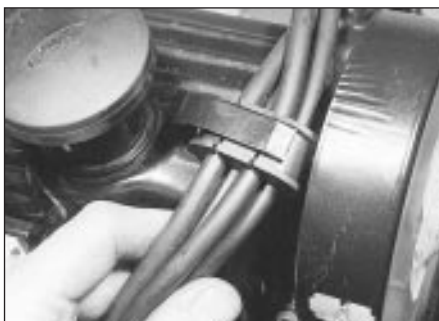
13.3 HT lead holder on camshaft cover
