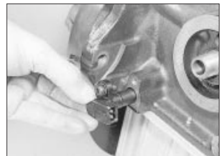
19.37 Removing the crankshaft speed/position sensor (engine removed)
