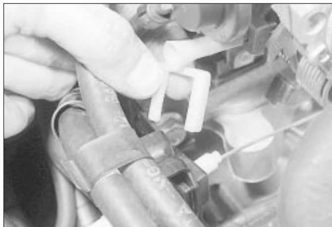
12.7 Removing the throttle cable sheath retainer securing clip - CVH model
