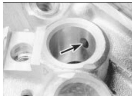
23.9b Cam follower supply hole (arrowed) in cylinder head - 1.8 litre (R2A)
