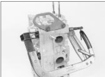
21.2a Compress the valve spring . . .
