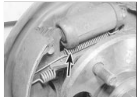
5.6a Top shoe return spring (arrowed)
