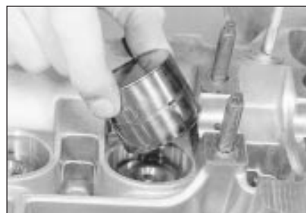
18.15 Withdrawing a cam follower
