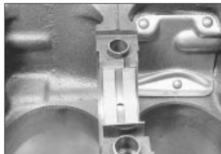
34.9 Extract each main bearing shell
