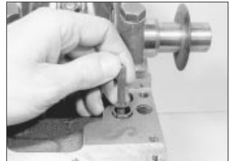
30.4 Withdrawing the oil pump driveshaft
