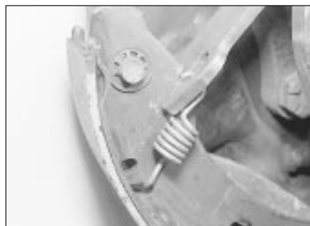
5.14 Strut and spring fitted to top of trailing shoe
