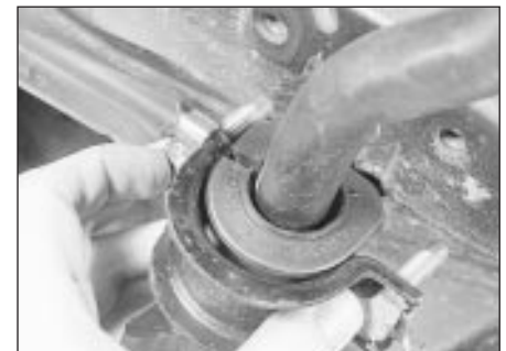
7.2b . . . unscrew the bolts and remove the anti-roll bar U-clamps
