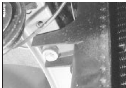
5.10b Lower radiator mounting bolt
