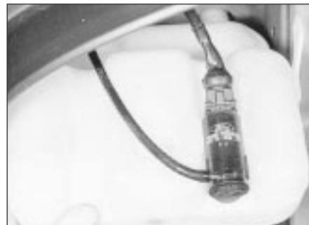
35.1 Windscreen washer pump - models from 1987
