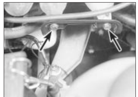
30.12 Lower inlet manifold bracket (arrowed)
