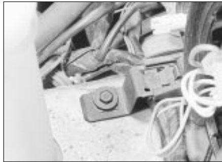
41.10a Remove the headlamp rear securing bolt . . .
