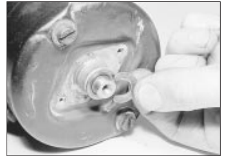
10.3a Remove the C-clip . . .
