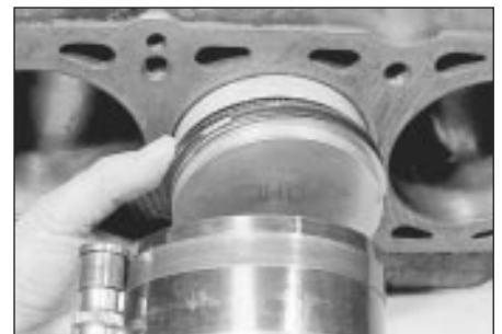
32.10 Fitting a piston ring compressor
