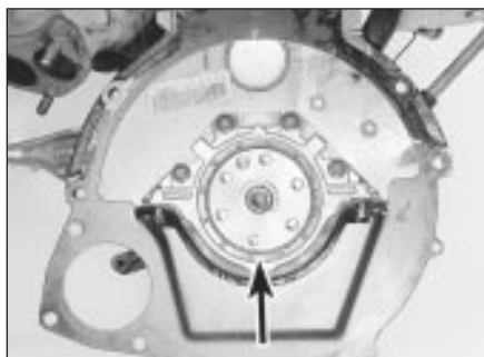
26.2 Crankshaft rear oil seal location (arrowed)
