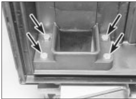
15.5 Airflow meter-to-air cleaner lid bolts (arrowed)
