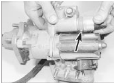
19.4 Refit the pressure switch with the drain hole (arrowed) in the plastic sleeve facing the pump motor - ABS
