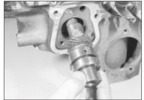
25.5b Withdraw the auxiliary shaft
