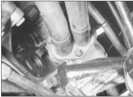
27.4a Exhaust downpipe-to-manifold flanged joint viewed from underneath vehicle
