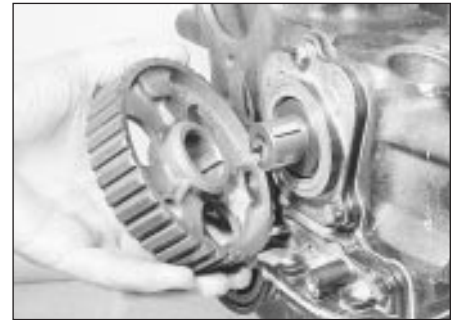
19.13 Removing the auxiliary shaft sprocket
