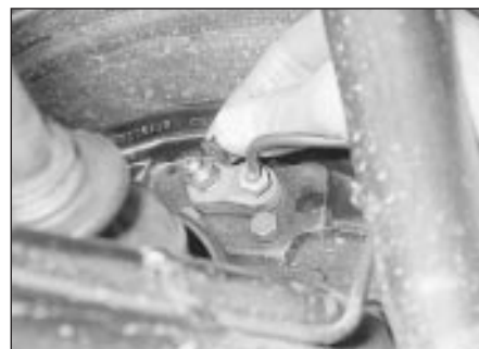
2.5 Removing the dust cap from a wheel cylinder bleed screw
