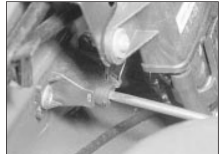
16.34b . . . to enable mixture adjustment - DOHC models
