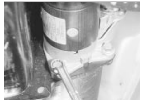
8.5 Unscrew the starter motor mounting bolts
