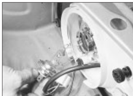
48.3b Release the spring clip and withdraw the headlamp bulb
