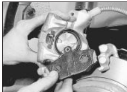
4.30 Lift out the disc pads
