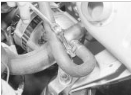
19.3a Disconnecting the heater coolant hose from the coolant pump elbow - 1.8 litre (R2A)
