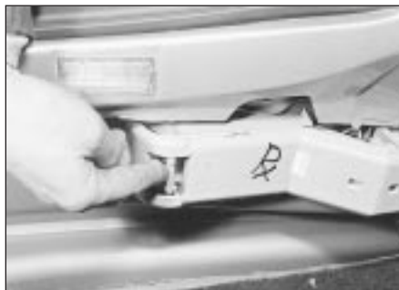
48.31a Press the plastic retaining tab to release the rear lamp bulbholder assembly - Saloon and Hatchback models
