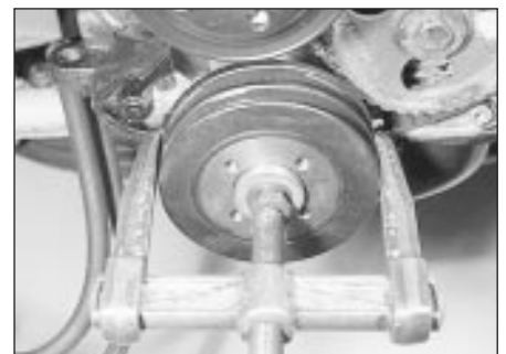
19.8 Using a puller to remove a pressed type crankshaft pulley
