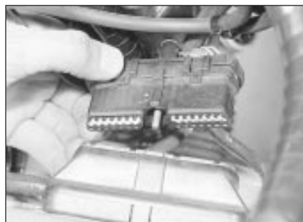
18.3c Disconnecting ESC Hybrid module wiring plug
