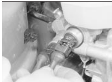
16.3b . . . the main valve multi-plug . . .
