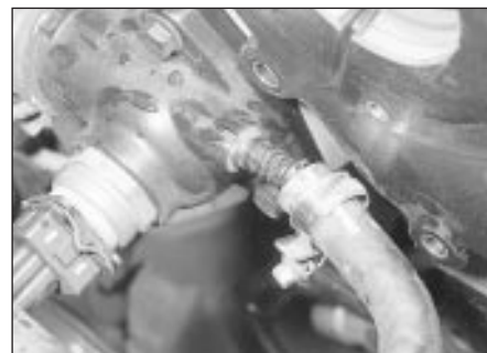
7.20a Disconnect the coolant hoses . . .
