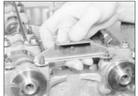
18.30c Fitting the timing chain guide plate
