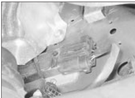
18.25 Ignition module location (arrowed)
