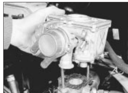
14.8b . . . and lift the carburettor from the inlet manifold - Ford VV carburettor
