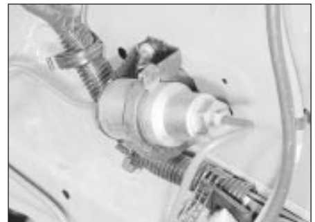
23.1b Later type deceleration sensitive valve
