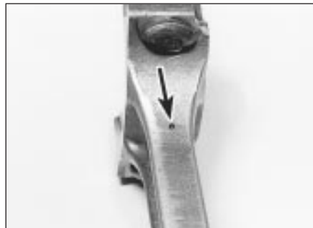
30.10c Connecting rod oil hole (arrowed) must face inlet manifold side of engine - 1.8 litre (R2A)
