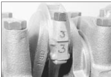
32.2 Big-end cap and connecting rod identification numbers
