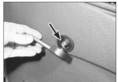
17.1b . . . then withdraw the window handle and bezel (arrowed)
