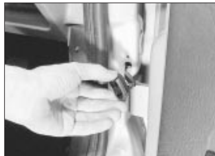
12.3 Withdrawing a courtesy lamp switch
