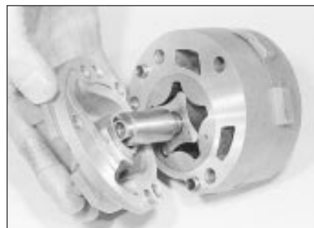
27.3 Removing the oil pump cover
