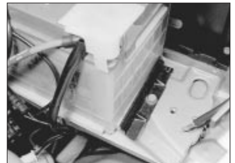
2.3 Battery securing clamp and bolt
