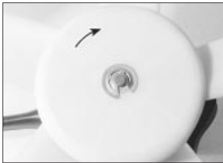
13.2 Fan blade securing clip and direction of rotation arrow
