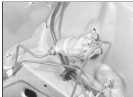
23.1a Early type deceleration sensitive valve
