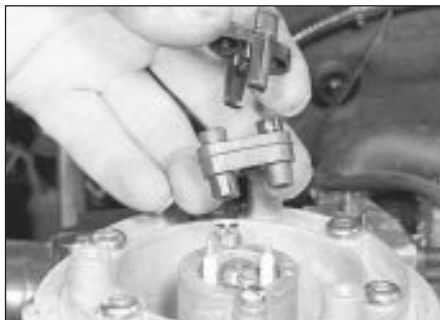
16.4 Disconnecting the fuel injector wiring plug
