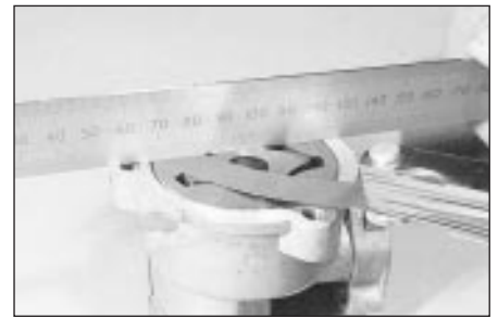
31.11 Checking the oil pump rotor endfloat
