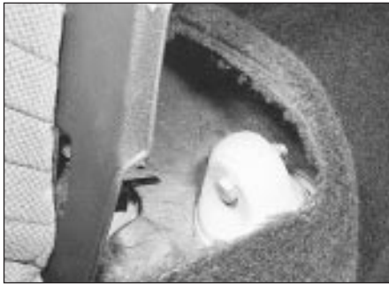
12.2b . . . for access to the rear shock absorber upper mounting
