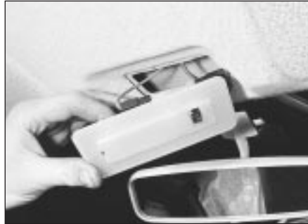
25.2a Removing a courtesy lamp
