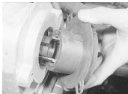
14.9 Removing the rotor housing
