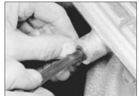
14.10 Disconnecting a later-type brake servo vacuum hose
