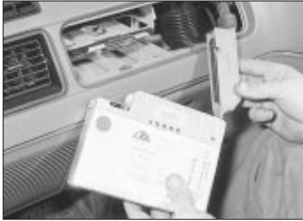
21.4 Withdraw the module and disconnect the multi-plug - ABS
