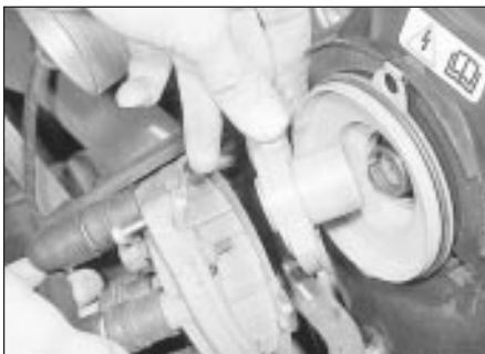
13.17 Removing the distributor cap and rotor arm
