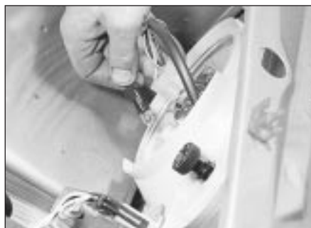
48.6 Removing a sidelamp bulbholder
