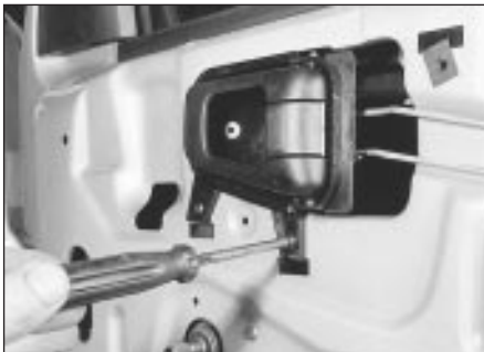
18.3a Remove the securing screws . . .
