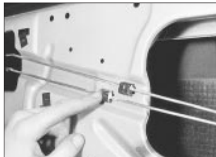
18.5 Remote control rods correctly located in their guides
