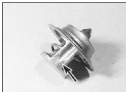
7.9 Thermostat flow direction markings (arrowed)
