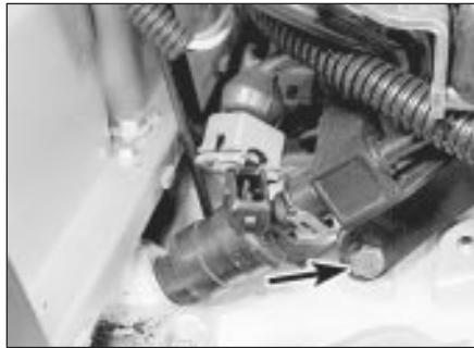
18.9a Fuel rail front securing bolt (arrowed) . . .
