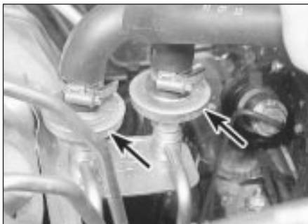
22.2 Pulse-air delivery check valves (arrowed)
