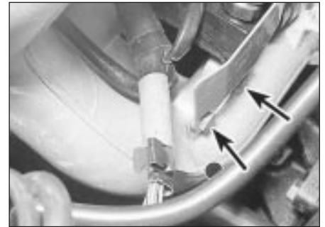
18.9b . . . and rear securing bolts
