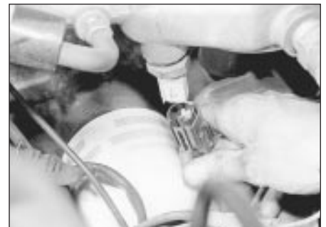
19.4 Disconnect engine temperature sensor wiring plug - ESC II system
