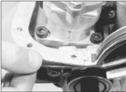
29.16 Locate the sump gasket end tabs beneath the rubber sealing strips
