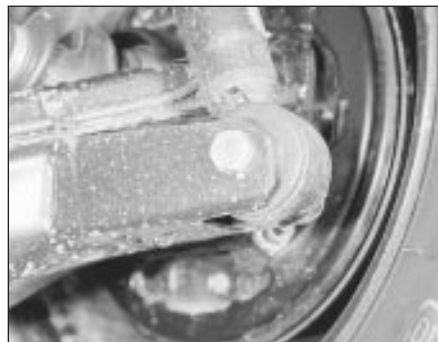
12.1 Rear shock absorber lower mounting - Saloon and Hatchback models
