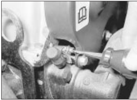
46.4 Unscrew the clip and remove the rubber cap from the bleed spigot - SOHC models
