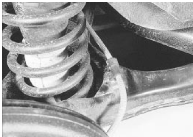
27.6 Handbrake cable-to-lower suspension arm attachment
