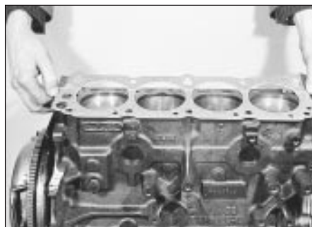
21.11 Fitting a new cylinder head gasket
