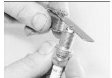
11.9a Measuring a spark plug gap using a feeler blade
