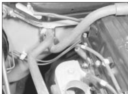
18.3 Location of heater hoses on engine compartment bulkhead
