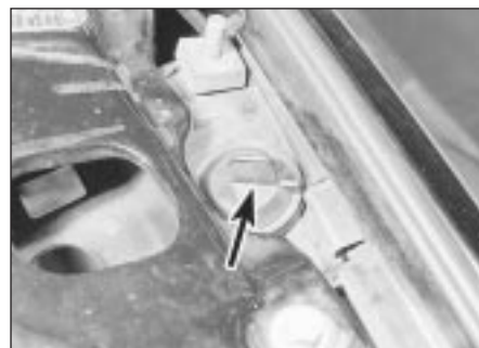
48.8 Auxiliary drive lamp bulb cover (arrowed) - models up to 1987
