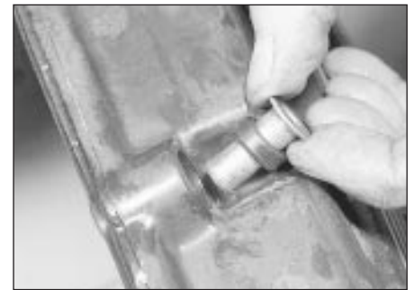
18.54 Fitting a camshaft cover reinforcing sleeve and sealing ring
