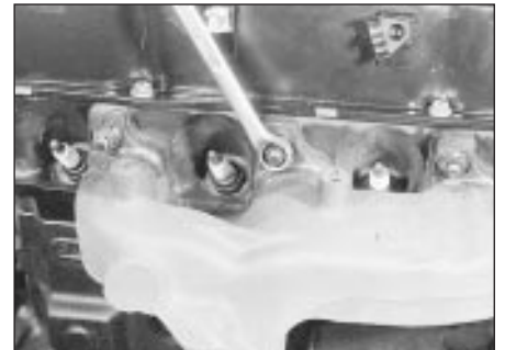
26.6a Unscrew the exhaust manifold securing nuts . . .
