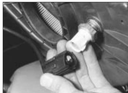
20.13 Disconnecting air charge temperature sensor wiring plug - ESC Hybrid system
