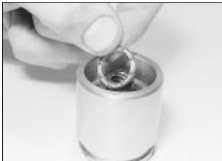
7.10d . . . then the thrust bearing . . .
