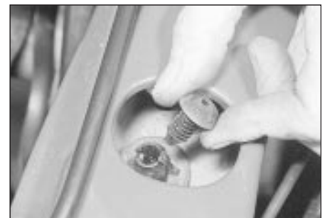
5.11 Removing a radiator upper locking peg
