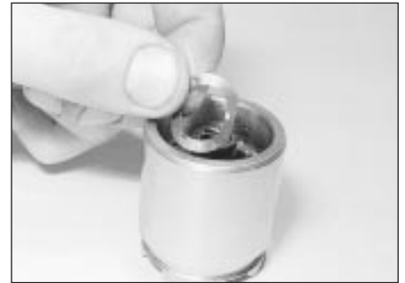
7.10c . . . a wave washer and (not shown) another thrustwasher . . .
