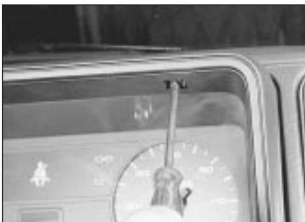
20.5 Removing an upper instrument panel surround securing screw
