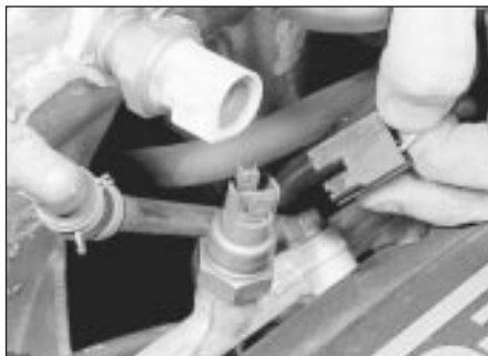
21.42 Disconnecting the fuel temperature sensor wiring plug
