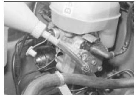
17.4 Topping-up the transmission fluid
