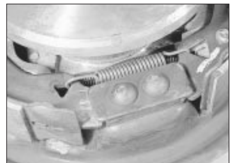
5.6b Bottom shoe return spring
