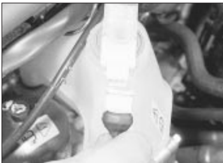
16.3a Disconnecting the low fluid level switch multi-plug . . .
