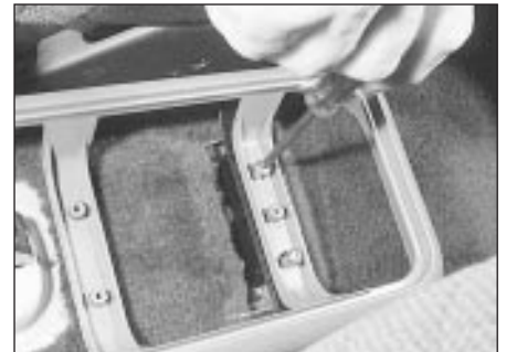
44.6c . . . and rear securing screw
