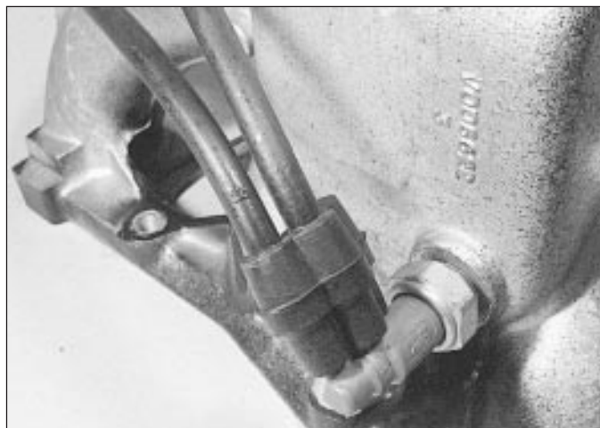
28.1 Low vacuum enrichment ported vacuum switch location in inlet manifold - model with Weber 2V carburettor
