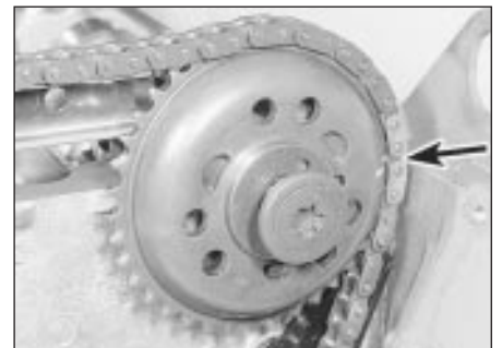
18.38 Spacer and sprocket securing bolt fitted to end of camshaft, with camshaft in TDC position (timing marks arrowed)
