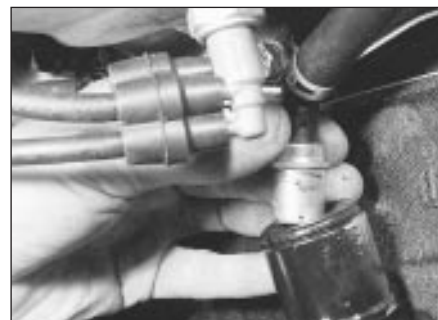
42.1 Removing the crankcase vent valve from the oil separator
