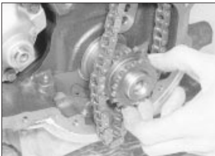
15.12 Sliding the double chain sprocket from the end of the crankshaft
