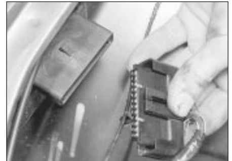
18.22 Disconnecting the ignition module wiring plug
