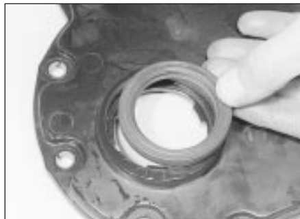
15.30 Fitting a new lower timing chain cover oil seal
