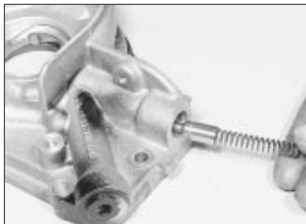
29.4 Unscrew the pressure relief valve plug and withdraw the spring and plunger
