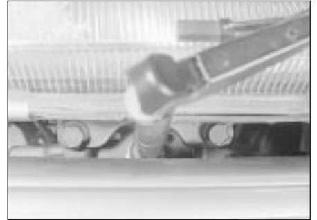
40.5b . . . for access to the headlamp wiper motor mounting bolts
