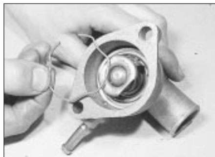
7.6a Prise out the retaining clip . . .
