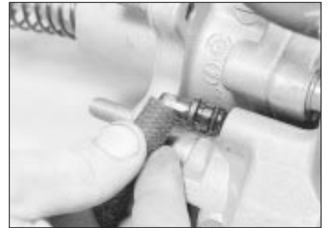
15.5b . . . and disconnect the low pressure fluid hose - ABS
