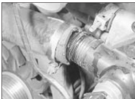
7.20b . . . from the thermostat housing
