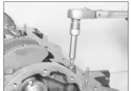
30.4 Unscrewing a sump mounting plate securing bolt
