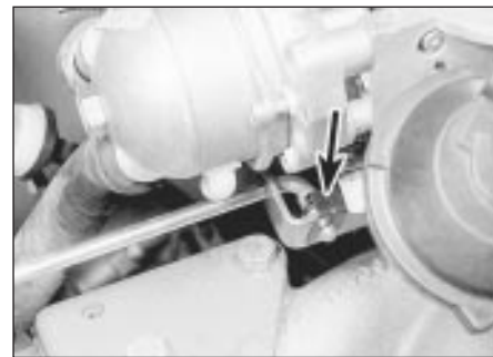
19.4 Throttle arm retaining clip (arrowed) - Pierburg 2V carburettor
