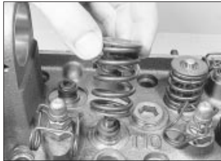
22.2b Removing a valve spring and cap
