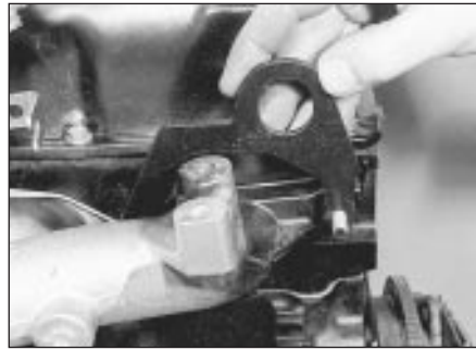
25.11 Rear engine lifting bracket location - SOHC models
