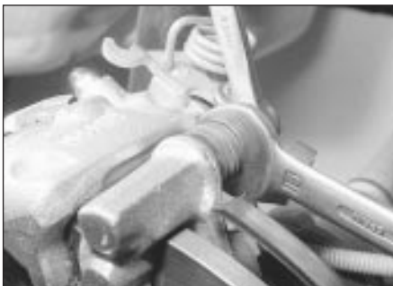
4.29 Unscrewing the forward caliper guide pin bolt
