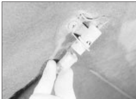
28.6 Removing an underbonnet lamp bulb
