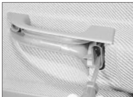
17.10b . . . and remove the armrest securing screws
