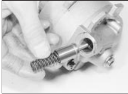
27.5b . . . and withdraw the spring and plunger
