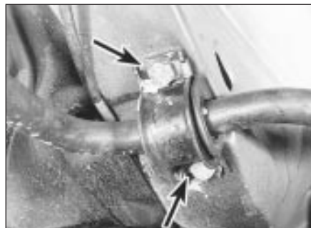
7.2a Bend back the locktabs (arrowed) . . .
