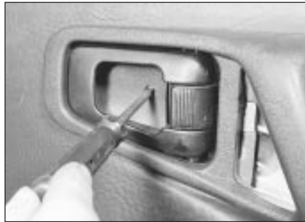
17.3a Remove the securing screw . . .
