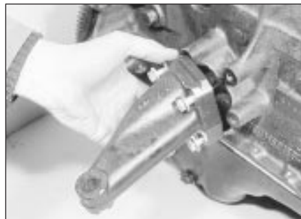
18.10a Removing the right-hand engine mounting bracket
