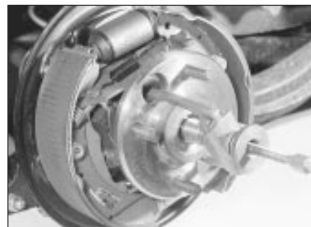
14.6 Pull the drive flange from the end of the driveshaft
