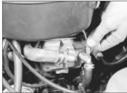
3.5 Disconnecting the air cleaner vacuum hose from the inlet manifold
