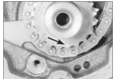
15.18 Coppered link in timing chain aligned with crankshaft sprocket timing mark (arrowed)
