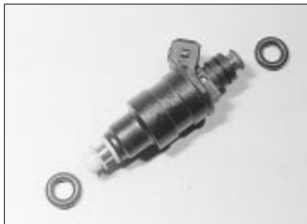
18.12 Fuel injector with seals removed
