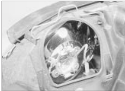
48.11 Auxiliary driving lamp bulb location - models from 1987
