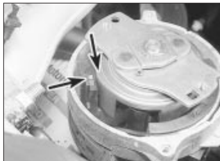
15.7c Trigger vane segment leading edge aligned with sensor rib - Motorcraft distributor
