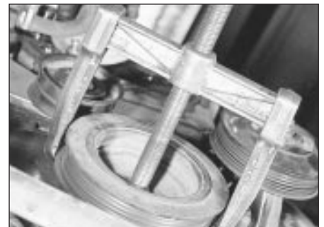
15.5a Remove the crankshaft pulley using a puller (viewed from under vehicle)
