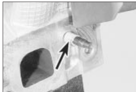
26.8b Remove the plastic spacer (arrowed) before fitting exhaust manifold gasket - CVH models
