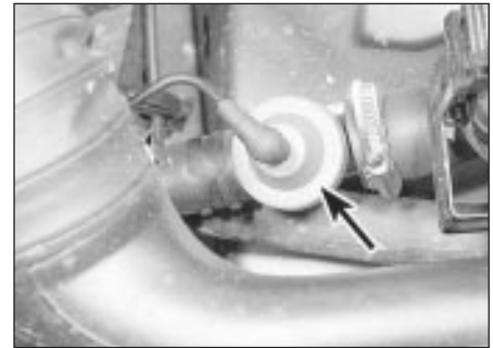
21.1 Pulse air system vacuum-operated air valve (arrowed)
