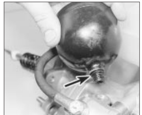
17.4 Unscrew the accumulator and remove it, noting the O-ring (arrowed)
