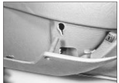
17.4 Withdraw the door pocket
