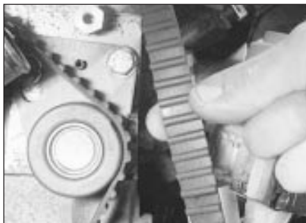
19.29 Twisting the timing belt to assess its tension
