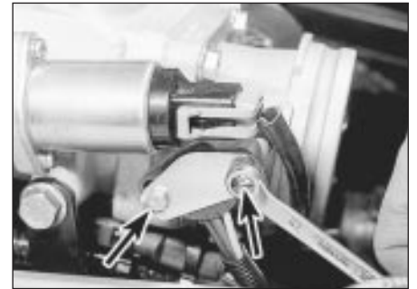
27.3 Unscrewing the throttle position sensor retaining bolts
