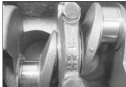
34.5 Main bearing cap identification marks. The arrow points to the front of the engine
