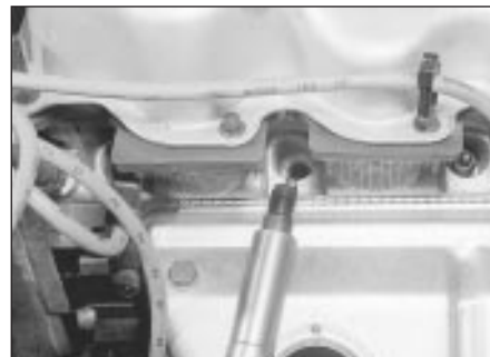
20.6 Removing a spark plug - CVH engine
