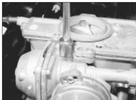
14.8a Remove the securing nuts and washers . . .
