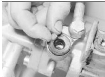
15.7 Removing the spigot locating bush from the rear hydraulic unit inlet - ABS
