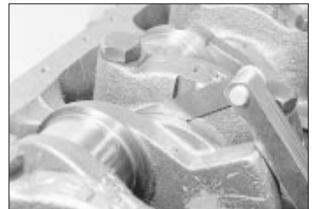
34.6 Checking crankshaft endfloat
