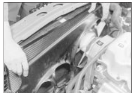
13.1 Withdrawing the fan shroud and cooling fan assembly
