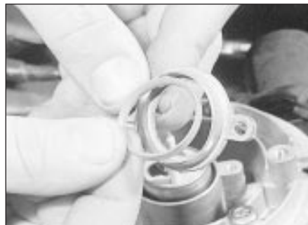
16.7 Removing the seal from the injector retaining collar
