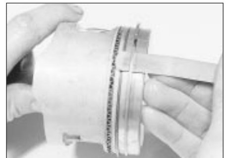
31.3 Using an old feeler gauge to aid the fitting of a piston ring - 1.8 litre (R2A)
