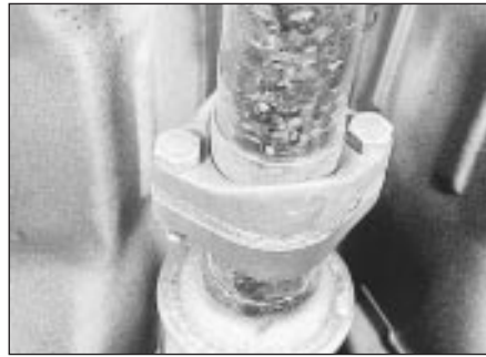
27.4b Exhaust downpipe-to-main system flanged joint
