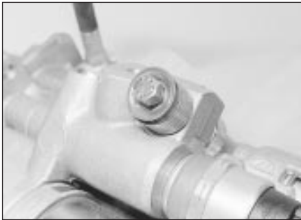
18.5 Hydraulic unit pump mounting bolt - ABS
