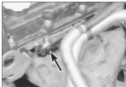
17.6 Hose bracket bolted to cylinder head (arrowed)
