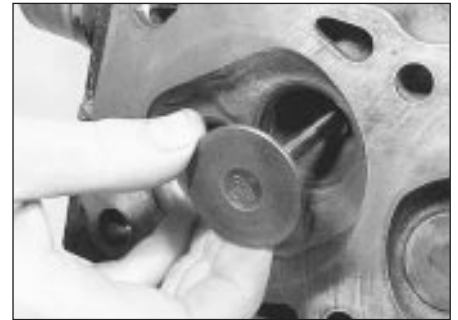
22.2c Removing a valve
