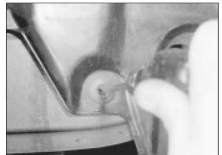
36.2 Releasing a wheel arch liner plastic clip
