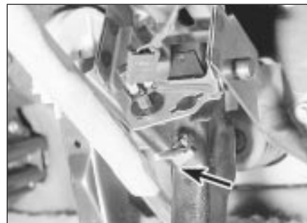
14.4 Remove the clip (arrowed) from the servo pushrod
