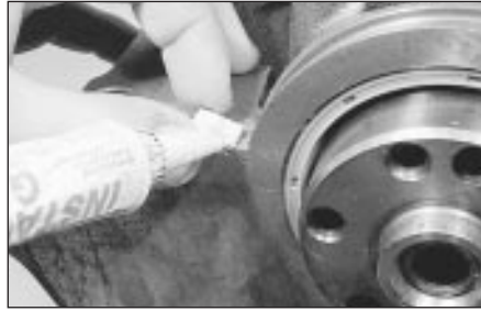
34.29 Fitting a sealing wedge to the rear main bearing cap
