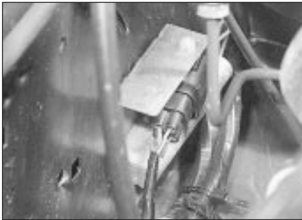
17.1 Fuel injector ballast resistor location (arrowed)
