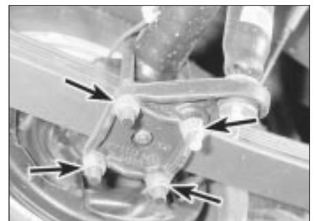
19.3 Unscrew the nuts (arrowed) from the rear axle-to-leaf spring U-bolts
