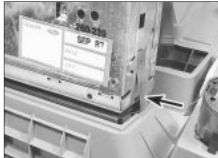
57.4 Radio/cassette player securing tangs (arrowed) viewed from the rear of the unit - standard fixing
