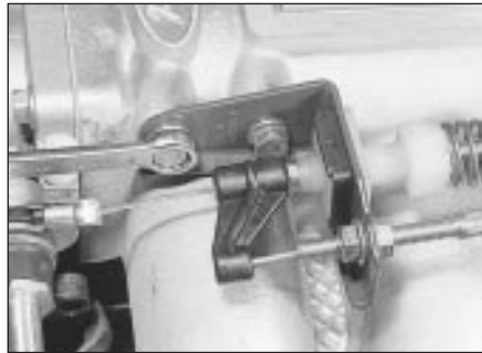
30.5 Unscrew the securing bolts and remove the throttle cable bracket
