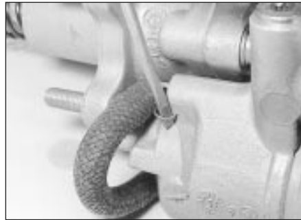
15.5a Remove the securing spring clip . . .
