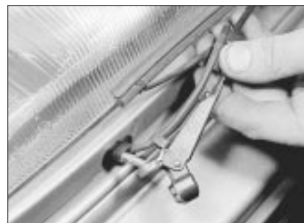
32.4 Removing a headlamp wiper arm
