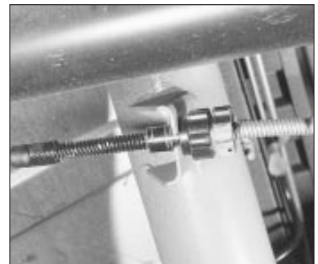
28.17 Handbrake cable adjuster on right-hand side of chassis crossmember
