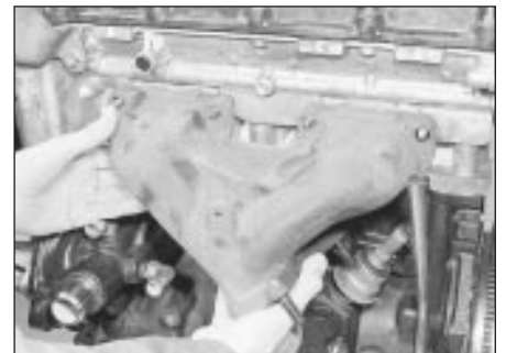
26.8c Fitting the exhaust manifold - DOHC models
