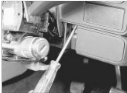
20.4b . . . for access to the lower right-hand instrument panel surround securing screw
