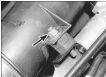
38.17 Air intake tube securing nut (arrowed)
