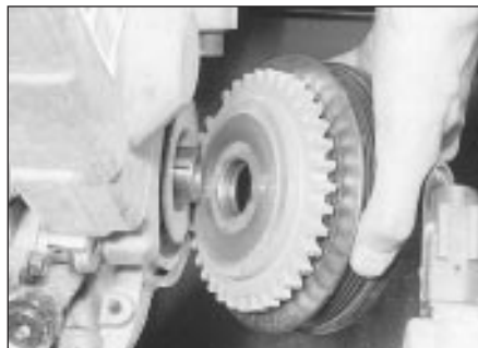
18.3 Withdrawing the crankshaft pulley - 1.8 litre (R2A)
