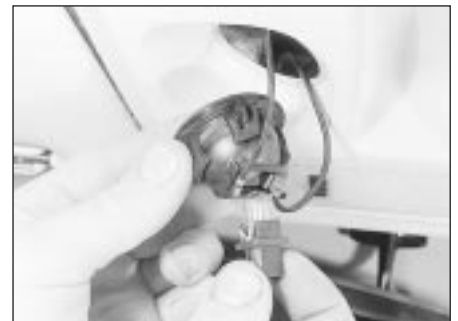
27.6 Removing a map reading lamp bulb
