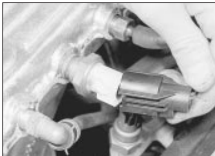
21.24 Disconnecting the air charge temperature sensor wiring plug
