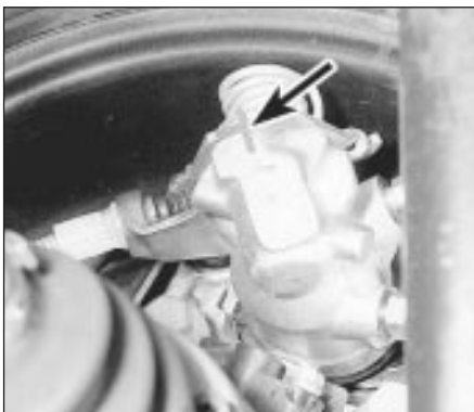
28.11 Make alignment marks between each handbrake operating lever and caliper body (arrowed) - ABS
