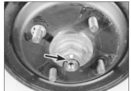
14.1b On early models relieve the staking (arrowed) on the rear hub nut
