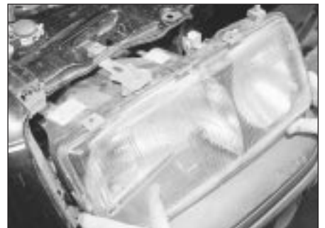
41.4d . . . then withdraw the headlamp unit - models up to 1987
