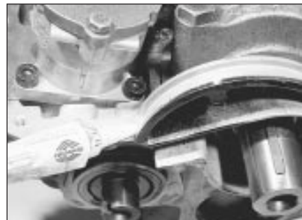
29.15a Apply sealing compound . . .
