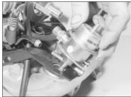
6.5 Withdrawing the fuel pressure regulator
