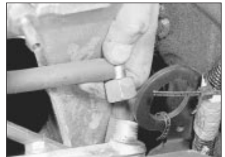
18.18 Disconnecting the fuel feed hose from the fuel rail
