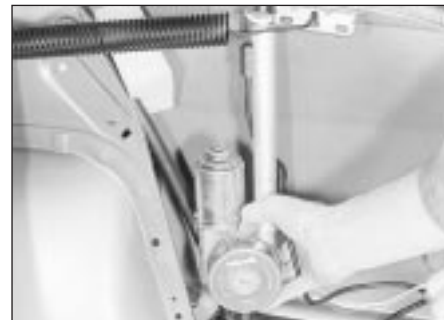
53.5 Removing an electric aerial - Saloon model
