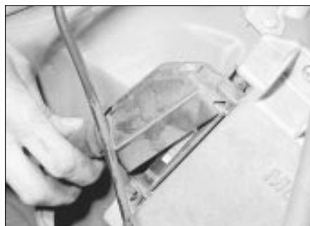
18.3b Disconnecting ESC II module wiring plug
