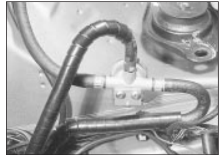
5.1 Fuel pressure regulator location - models up to 1985
