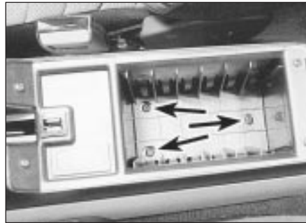
44.3b Rear upper console panel rear retaining screws (arrowed)
