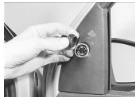
29.1 Unscrew the bezel from the adjuster knob . . .
