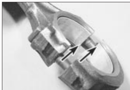
32.8 The bearing shell lugs (arrowed) must be adjacent to each other
