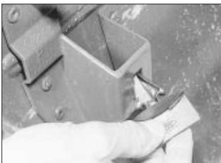
30.15 Rear bumper plastic fastener
