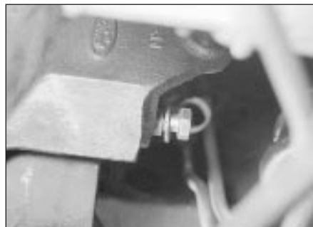
29.14b Power steering pump rear securing bolt
