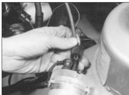
12.7 Disconnecting the HT lead from the coil
