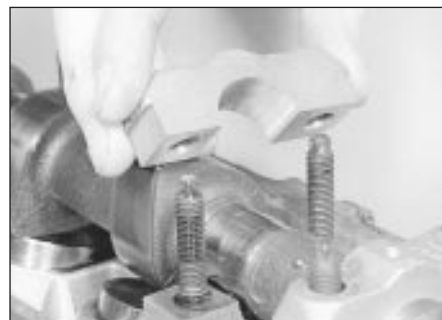
18.14a Lifting off a camshaft bearing cap
