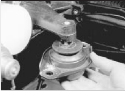
17.4 Withdrawing an engine mounting
