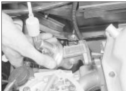
8.4 Withdrawing the fuel pump from the cylinder head - CVH model
