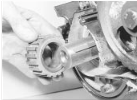
19.11 Removing the crankshaft sprocket
