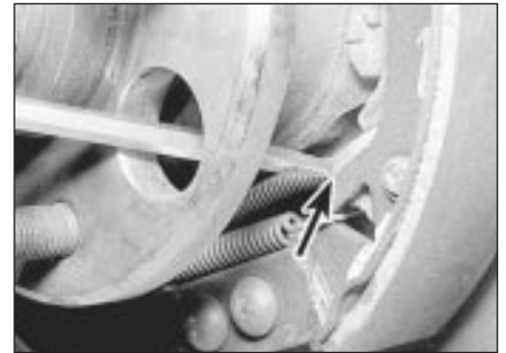
5.5c Drum removed showing screwdriver pressing on adjuster ratchet
