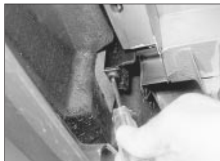
30.18 Adjusting the height of a rear bumper
