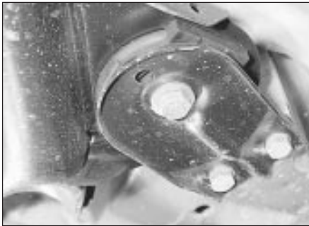
11.10 Rear suspension front guide plate
