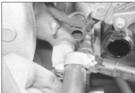
17.5 Disconnecting the heater coolant hose from the inlet manifold
