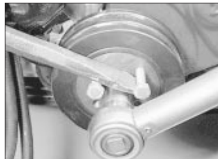
19.33 Holding a pressed type crankshaft pulley with two bolts and a lever while tightening the bolt
