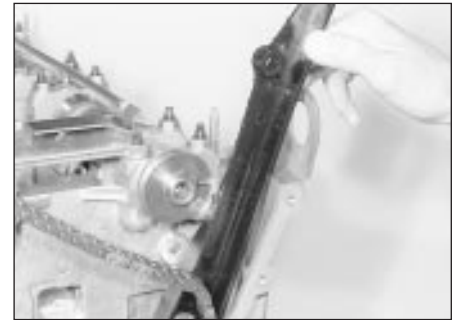
15.11 Withdrawing the lower timing chain guide
