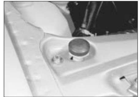
6.9 Adjustable bonnet rubber bump stop
