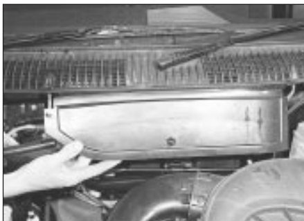
20.4 Unscrew the securing bolts and withdraw the heater motor cover
