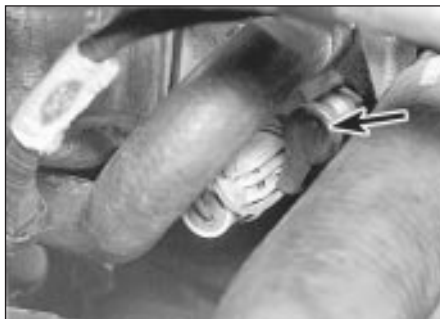
16.1 Temperature gauge sender location (arrowed)
