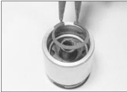
7.10a Remove the circlip from the rear caliper piston . . .
