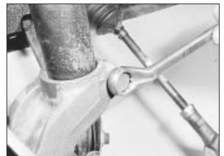
5.8 Unscrewing the hub carrier-to-strut pinch-bolt
