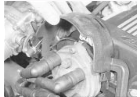
13.14b . . . and the upper section of the distributor shield
