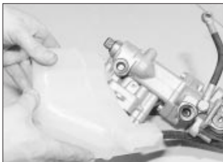
15.6 Removing the fluid reservoir from the hydraulic unit - ABS
