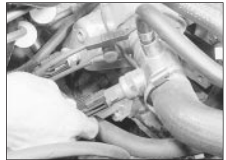
14.1 Disconnecting the wiring plug from the cooling fan switch
