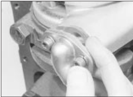
28.5 Removing the oil pick-up tube from the oil pump
