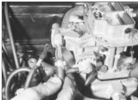
14.6 Disconnecting the fuel hose - Ford VV carburettor
