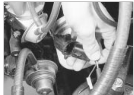
15.8 Disconnecting distributor wiring plug - Bosch distributor
