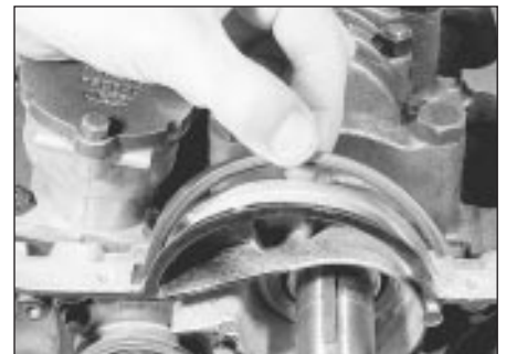
29.15b . . . then fit the rubber sealing strips
