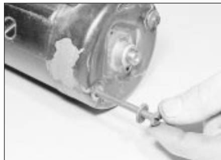
10.4a Remove the commutator end housing securing screws - Bosch long frame starter motor
