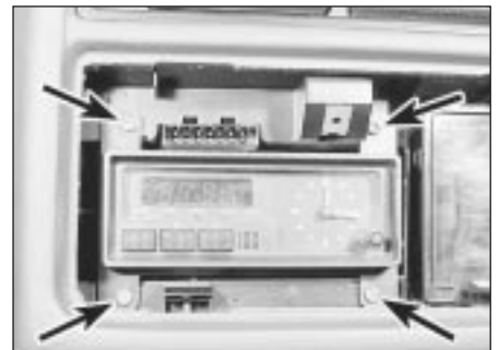
19.6 Multi-function digital/analogue clock securing screws (arrowed)
