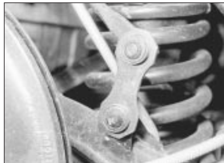
17.2 Anti-roll bar-to-lower arm connecting strap
