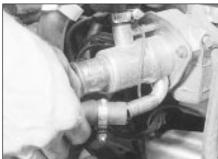
7.12a Disconnect the automatic choke hose . . .
