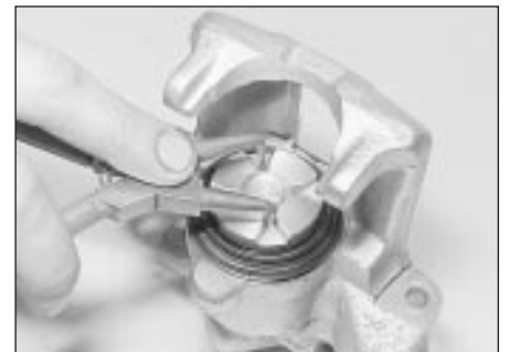
4.32 Retracting the piston using circlip pliers
