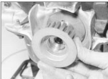
18.10a Remove the crankshaft sprocket ...
