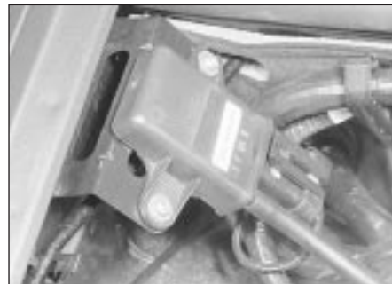
21.35 Manifold absolute pressure (MAP) sensor location
