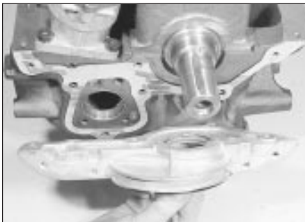
27.3a Removing the crankshaft front oil seal housing
