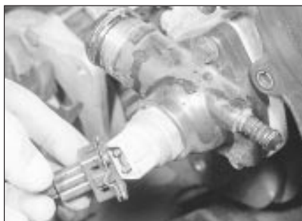
7.21 Disconnect the cooling fan switch wiring plug
