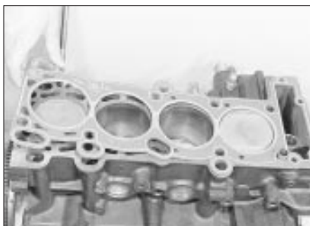
18.22 Fitting a new cylinder head gasket
