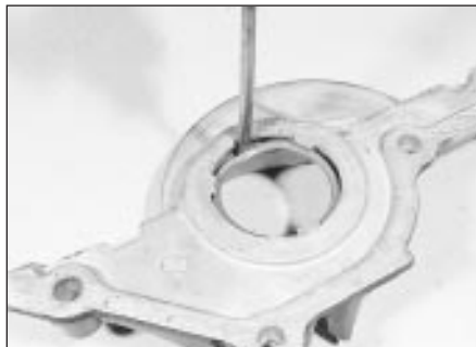
27.3b Driving the crankshaft front oil seal from the housing
