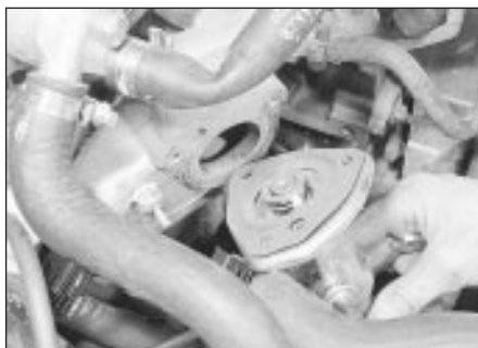
7.13 Removing the thermostat housing and gasket
