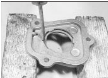
25.9a Driving out the auxiliary shaft cover oil seal
