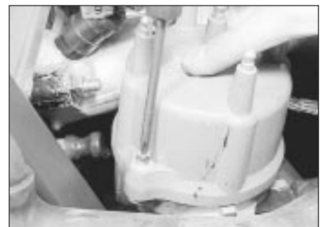
13.10 Removing a distributor cap securing screw - Motorcraft distributor
