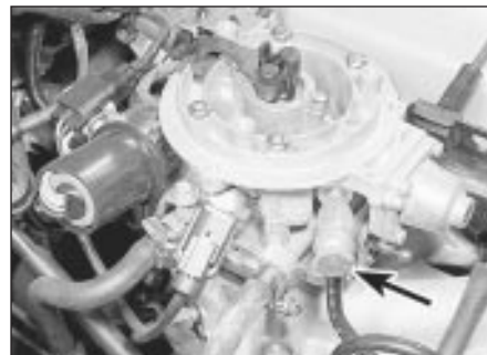
4.4 CFI unit fuel inlet union (arrowed)
