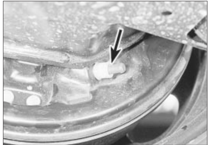
28.5 Plastic plunger (arrowed) in brake backplate
