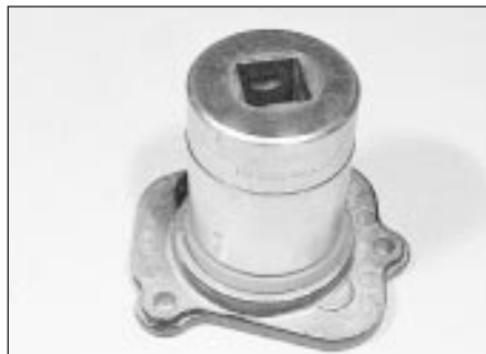
25.9b Using a socket to fit a new auxiliary shaft cover oil seal
