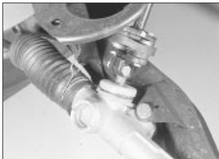
26.3 Intermediate shaft-to-steering gear flexible coupling
