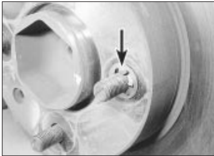
5.5a Brake drum retaining spire washer (arrowed)
