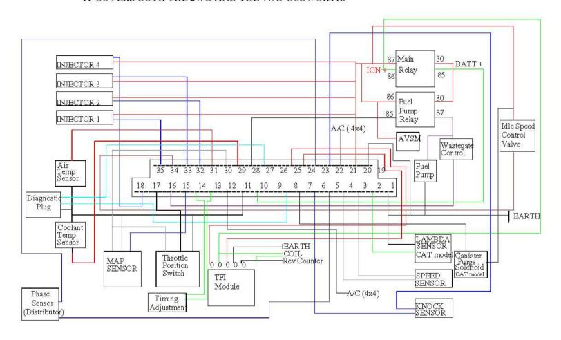
**EARTH** TERMINALS 1 AND 19. CHECK MAXIMUM OF 0.5 VOLT DROP BETWEEN TERMINAL AND BATTERY NEGATIVE.
