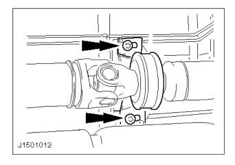
7. Detach the driveshaft intermediate bearing.
