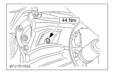
40. Tighten the torque converter bolts in the engine drive plate.
