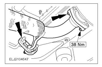
48. Attach the front exhaust pipe to the rear exhaust pipe.
