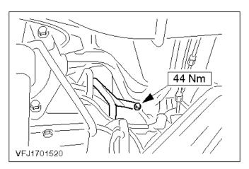
42. Install the oil filler pipe bracket on the transmission flange.
