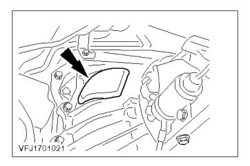
41. Install the torque converter housing cover.
