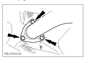
10. Detach the front exhaust pipe from the exhaust manifold.
