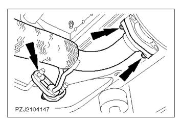
12. Remove the front exhaust pipe.
