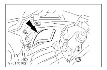
19. Detach the torque converter housing cover.
