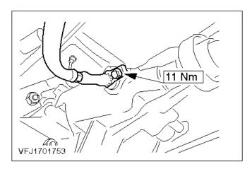
47. Install the speedometer drive gear.
