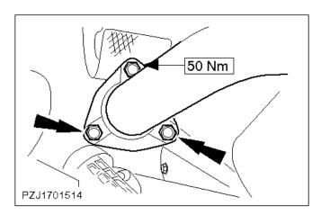
50. Install the front exhaust pipe on the exhaust manifold.
