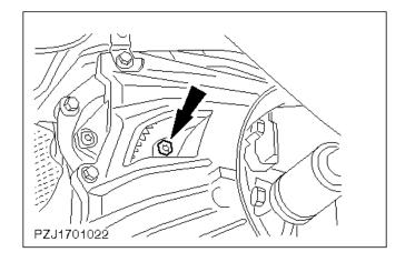
Unscrew and remove the torque converter bolts from the engine drive plate.
