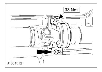
53. Install the driveshaft intermediate bearing.
