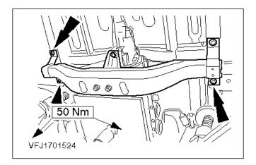
µ 37. Attach the transmission crossmember to the transmission and the bodywork.
