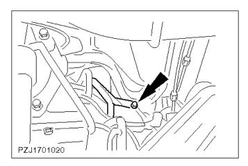
18. Detach the oil filler tube from the transmission flange.
