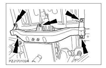
${f \mu}$  24. Detach the complete transmission crossmember from the transmission and bodywork.
