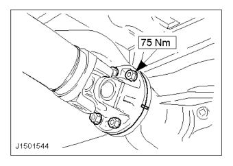
□ 51. Slide the driveshaft into the automatic transmission.
