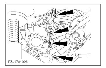
26. Unscrew and remove the transmission flange bolts on the left-hand side.
