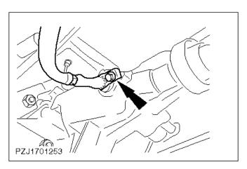
13. Detach the speedometer drive gear.
