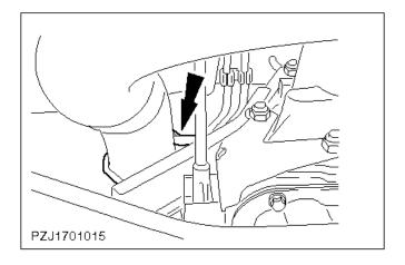
11. Detach the front exhaust pipe from the bracket (one nut and bolt).
