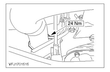
49. Install the front exhaust pipe on the bracket (one nut and bolt).
